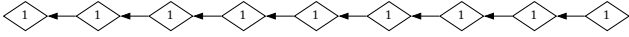
Fig. 1: Example chain for sequential proof-of-work. Each diamond represents one block. Arrows indicate hash-references. The labels show the constant incentive scheme: each proof-of-work gets the same reward.
